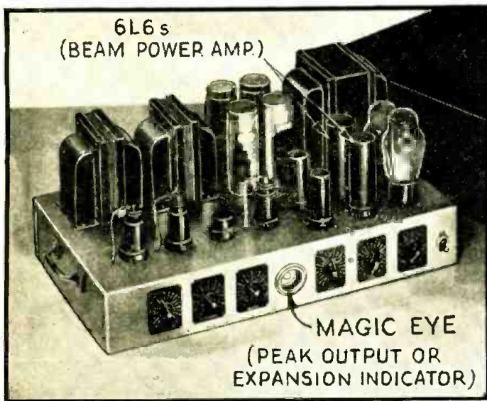
Fig. A. The appearance of the amplifier chassis.
