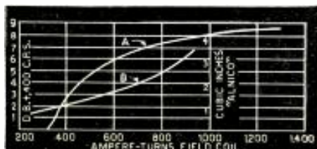
Fig. 1. Comparison of coil and alnico fields.
