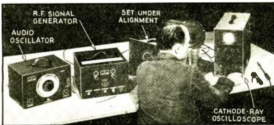
A modern set-up—the instrument on the cover would supplement the modern oscilloscope at the right.
